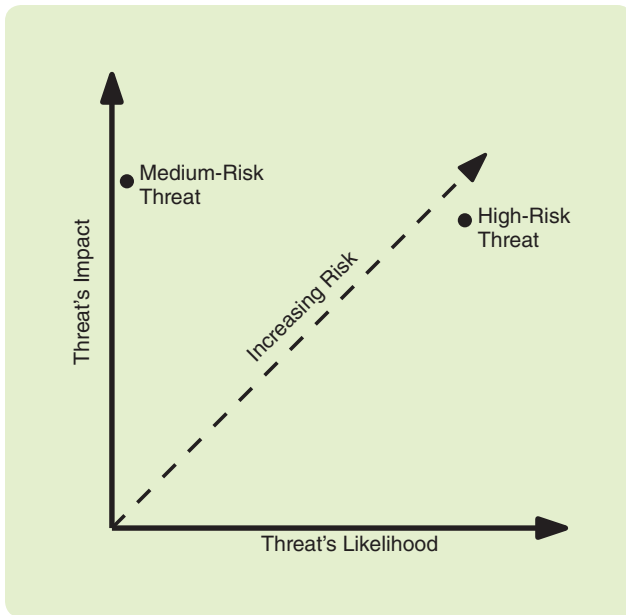
FIGURE 5 A risk matrix plot. The threat's likelihood and impact correspond to the x axis and y axis, respectively. Two threats with a similar impact but different likelihoods are depicted. Threats with high impact and high likelihood yield a higher risk.
