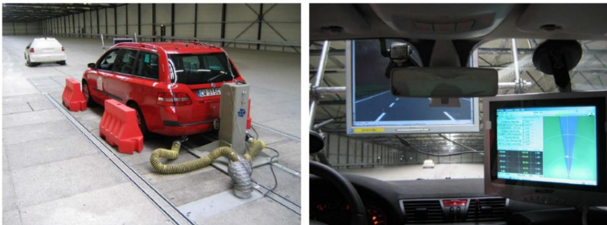
Figure 2.4: VeHIL testing laboratory [2]
